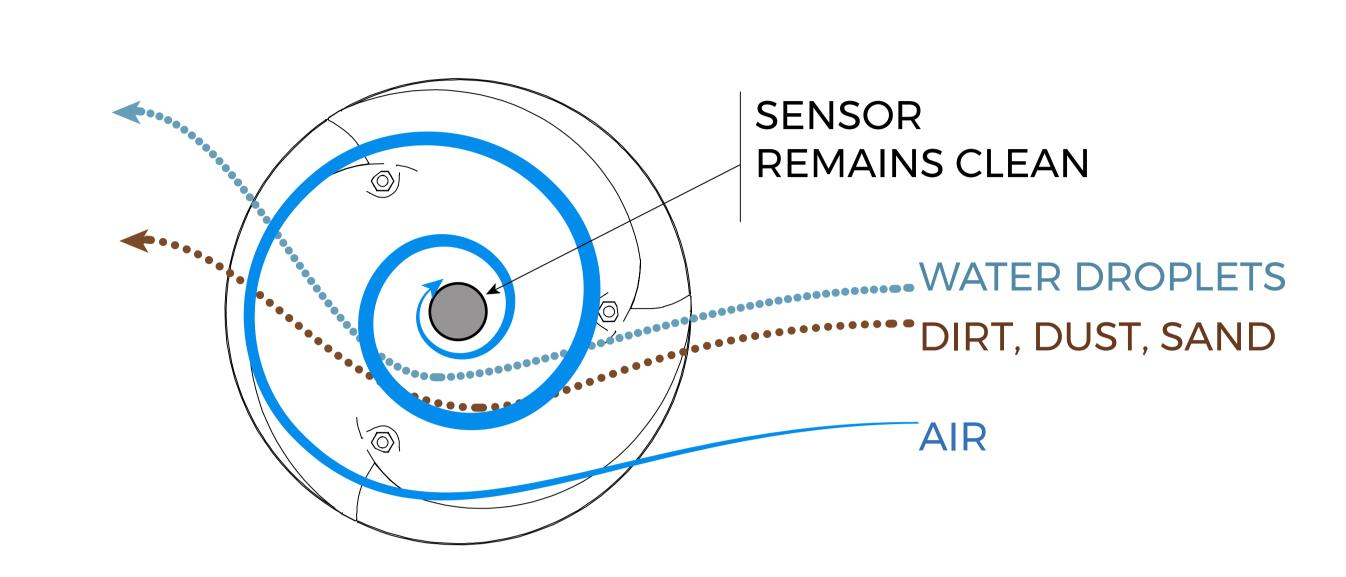
HEAVIER THAN AIR PARTICLES LIKE DIRT, DUST, SAND & WATER ARE PUSHED AWAY FROM THE SENSOR BY CENTRIFUGAL FORCES OF THE SPIRAL FLOW
